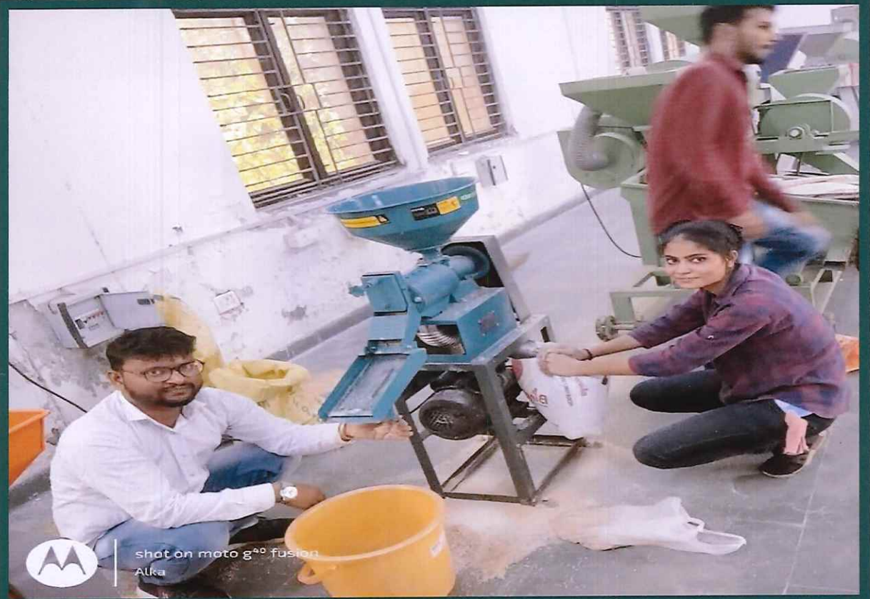
Experiential learning students of the university shelling rice on Rice sheller at Agro processing centre
